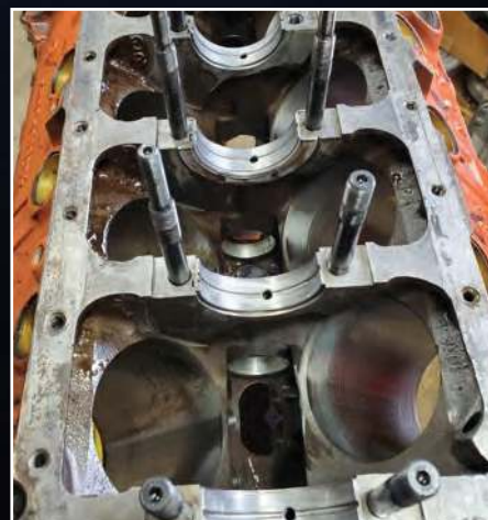
After 13 years of drag racing, the bearings in Jordan's Chrysler 408 showed virtually no signs of wear.
