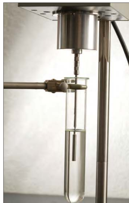
Viscometer device used to determine a liquid's absolute or kinematic viscosity.
