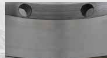
The transmission output shaft bearing showed no scoring, spalling or corrosion following 500,000 miles with AMSOIL Long-Life Synthetic Transmission Oil.
