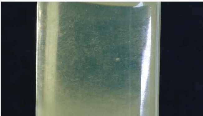
Wax crystals in untreated diesel fuel. The wax crystals will eventually fall out of solution and plug the fuel filter.
