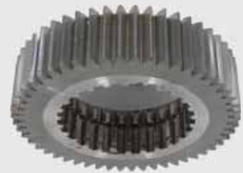
After 500,000 miles of real-world service, the transmission mainshaft input drive gear lubricated with AMSOIL Long-Life Synthetic Transmission Oil showed minimal wear and is suitable for continued use.
