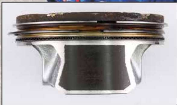
The piston skirt contained no scuffing and appears like-new, while the piston crown demonstrated no abnormal deposits following 100 severe-service hours.
