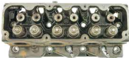
Cylinder head after cleanup with AMSOIL Engine and Transmission Flush. The valve springs and push rod openings are noticeably cleaner, with fewer sludge deposits. The manufacturer's stamping is more easily seen.
