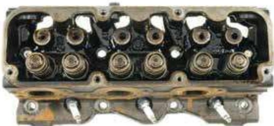
Cylinder head pre-cleanup. Note the sludge deposits on and around the valve springs and push rod openings.
