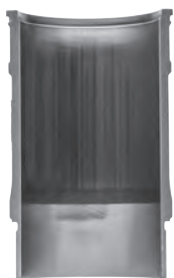
Severely Scuffed Liner
