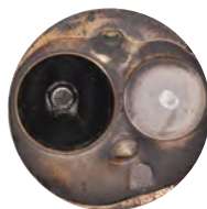
Cylinder head after one P.i. treatment.
