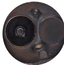
Cylinder head before P.i. treatment.
