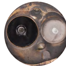
Cylinder head after one P.i. treatment.
