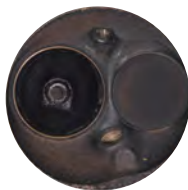
Cylinder head before P.i. treatment.
