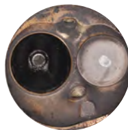
Cylinder head after one P.i. treatment.
